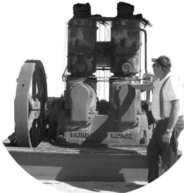
1917 80HP Fairbanks-Morse Diesel Engine
